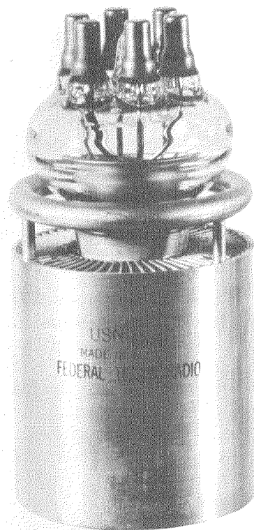
Fig. 32— 7C23 forced-air-cooled triode used in radar service.
