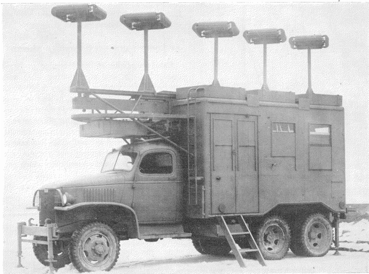
Fig. 3—Localizer truck for the SCS-51 portable instrument landing system used by the Army Air Forces.
